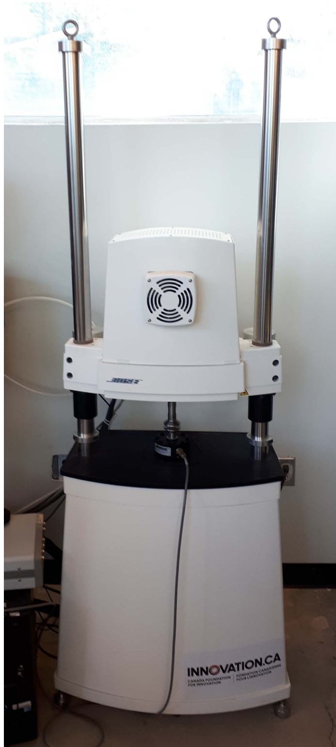
Figure 3.21: a) A photograph of the equipment used for the measurements (Bose Electro-Force 3300 Series II).
