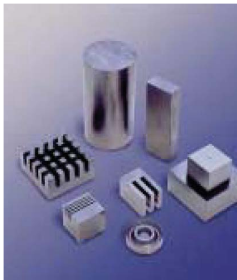
Figure 1.7: Photographs of products manufactured from compression molded graphite/epoxy composite. The figure has been reprinted from Norely et al. [33]. ©2001 IEEE.
