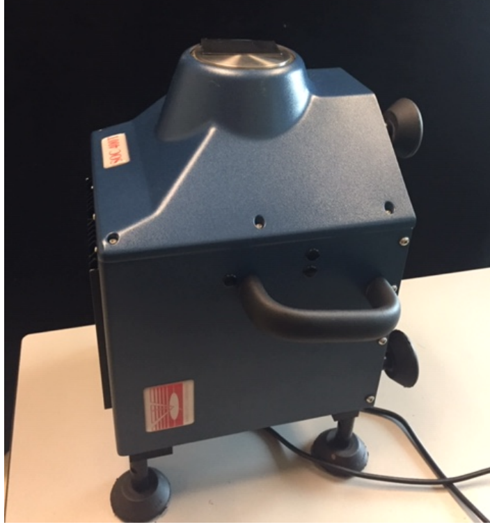
Figure 3.64: A photograph of a Surface Optics Corporation 400T Fourier Transform Infrared Reflectometer that was used for measuring the emissivity.
