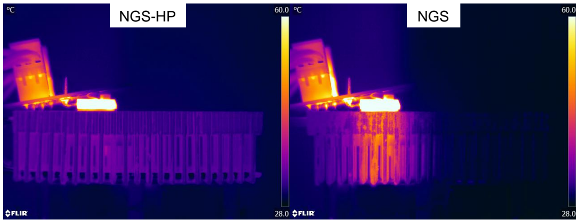
Figure 5.21: Infrared camera images of NGS+HP (left) and NGS(right) heat sinks
